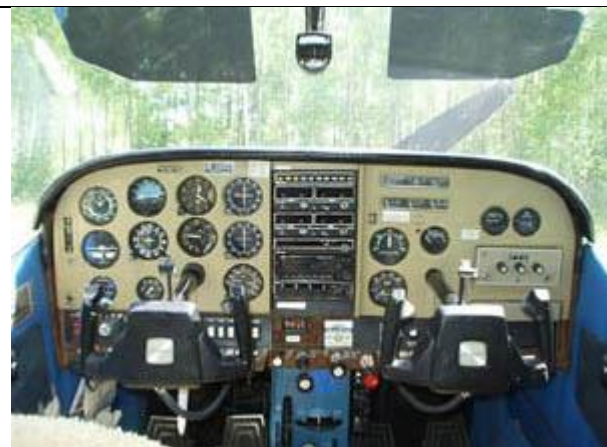
Glare Shield shown above is for 1975 Cessna 182 (Part No. SA39-1823) - Some modification on customer's part needed for proper fit.
