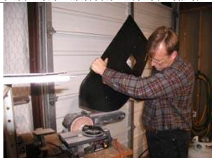
Bill final trims on belt sander to get to trim line and produce a smooth finish.
