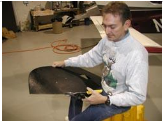
Step 4: Randy accomplishes gross trimming with shears to remove excess material.
