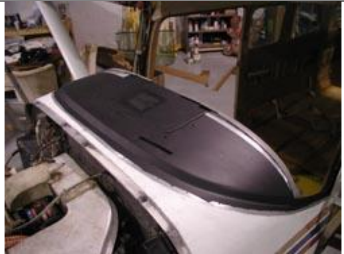
Step 2: The radio access plate was reinstalled.
