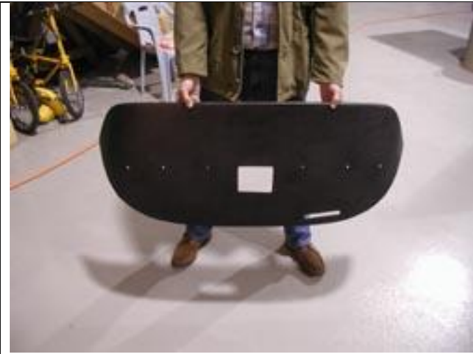
Unit ready for install with all trim and penetrations accomplished.
