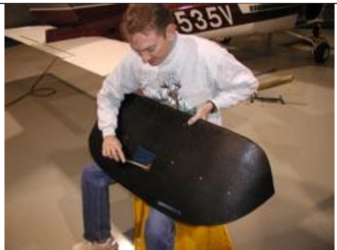
Randy performing detail trimming for speaker and defroster holes.
