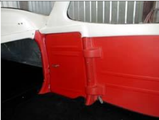
Left side view of 1978 Cessna 172. Note large hinge on front baggage door fairing.
