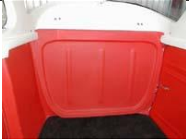
Rear view of Cessna 172. Note fuselage cover part no. SA60-14 to close off tail of the airplane.
