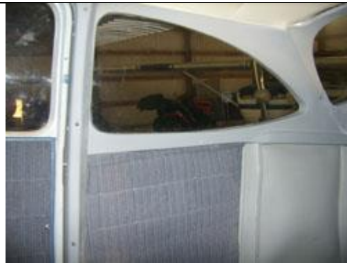
Part number SA60-16 in early 1960s vintage Cessna 172. Lower panels are original pieces covered in fabric.
