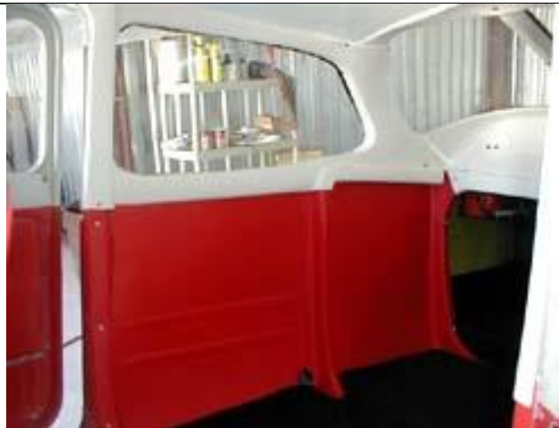
Right side view of 1978 Cessna 172. Note the shape of the side window part no. SA60-16-1.
