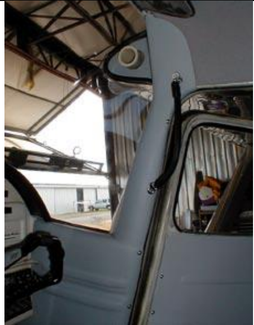
Front door post SA55-02 for early style Cessna 170, 172, 180, and 182 aircraft. The hand hold strap is secured in with screws.
