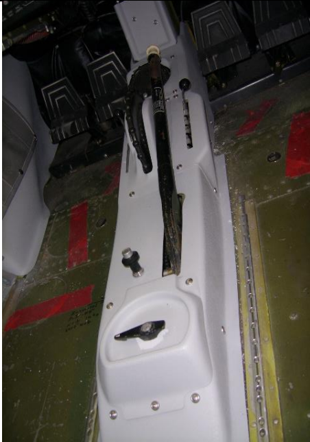
Flap tunnel cover with late style SA55-22 fuel selector cover, cowl flap handle cover SA55-26, trim control wheel cover SA55-20 and yoke control shield SA55-23.
