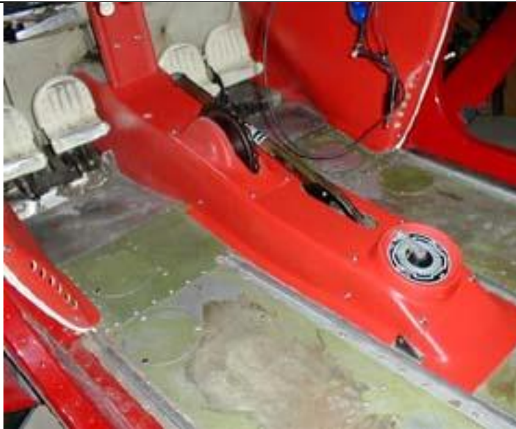
Flap tunnel cover with round fuel selector cover for early C170, 172, 175 and 180 models. Note elevator trim control wheel cover and yoke control shield cover.
