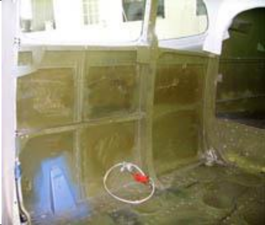
These 2 pictures show a bare side wall of aircraft (L) and (R) the after photo of the 1/2" black closed cell rubber soundproofing installed. We recommend a spray-on 3M adhesive and touch of contact cement. We provide a burn test for all rubber soundproofing sold. We sell ceiling and extended bag rubber soundproofing kits for many Cessna 170-206 aircraft. 1/4" rubber also available.
