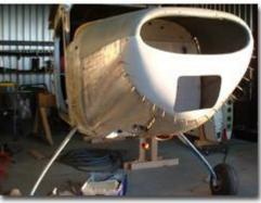
4.) This picture shows the clekos on the lower SA40-04 nose bowl before removing off the airplane and riveting into place.
