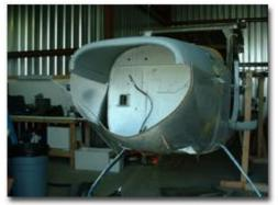
1.) Remove the doubler strips. Place in spacers underneath, on half that is hooked to cowling. Then place doubler strips back onto the cowling.
